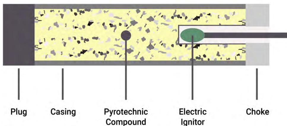
A plug placed at one end of the container with a small orifice, called a choke, constricts the expulsion of the ignited pyrotechnic compound, increasing the size and aggressiveness of the jet.
