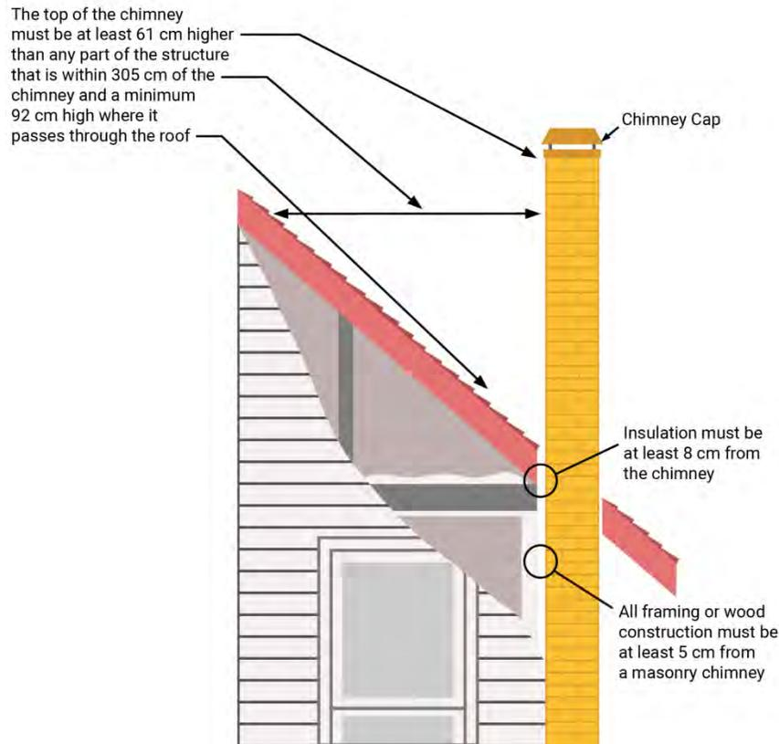
The science behind the workings and the function of chimneys is also very interesting. As mentioned previously, chimneys basically help remove all the byproduct gases from the air. Every fireplace requires a chimney because there has to be an outlet for the transfer of heat, gas, and smoke. One of the biggest cornerstones for any chimney is 'airflow' without which it wouldn't exactly be functional.
