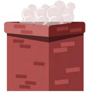
All the heat and smoke passes upwards through a tunnel-like channel to the roof and then out into the atmosphere. An interesting feature of this type of chimney is that often the bricks that are used in its construction have the ability to absorb heat. This comes in really handy, especially during the winter season as some of the absorbed heat radiates to other rooms and keeps them warm.
